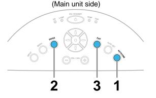
A picture may be expanded on the upper side if projected upward from the projector lifted up by the foot adjuster. The projector can correct this keystone distortion.
